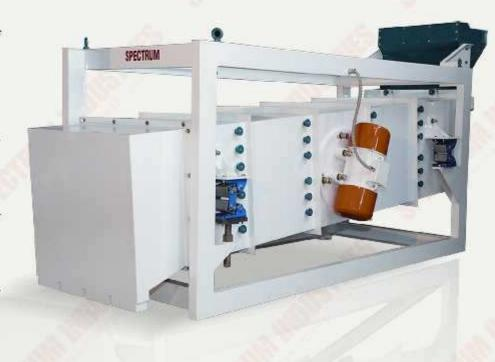
The screens can easily be changed by swinging down the inlet door and sliding them out
